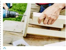
Step 7: Apply some glue on the end of a leg and position roughly in the centre of the pilot hole. Using the 75mm screws, fasten to seat with either a battery drill or screw driver. Repeat for all four legs. »
