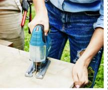
Step 3: Using a jigsaw, cut around the shape. Remember to wear safety equipment such as glasses and ear protection. Repeat for second stool.
