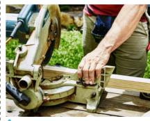
Step 5: Using a drop saw or a hand saw, cut four lengths of the 42 x 42mm pine for each stool to about 250mm. These
